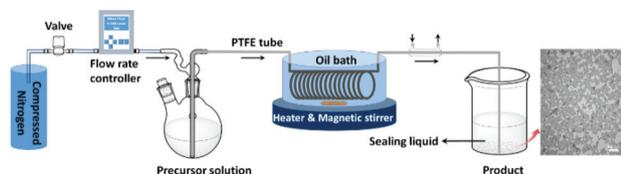
**Fig. 1** Schematic illustration of an inert-gas-driven microflow reactor for continuous synthesis of nanocrystals. The last panel shows a representative TEM image of as-synthesized  $\text{Cu}_2\text{S}$  nanocrystals, and the scale bar is 100 nm.
